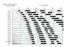
4. Go to the field and collect your data. Pick breaks quickly and accurately with the automated picker and adjust them manually with an interactive cursor. View travel times from other shots simultaneously for best coherence.
