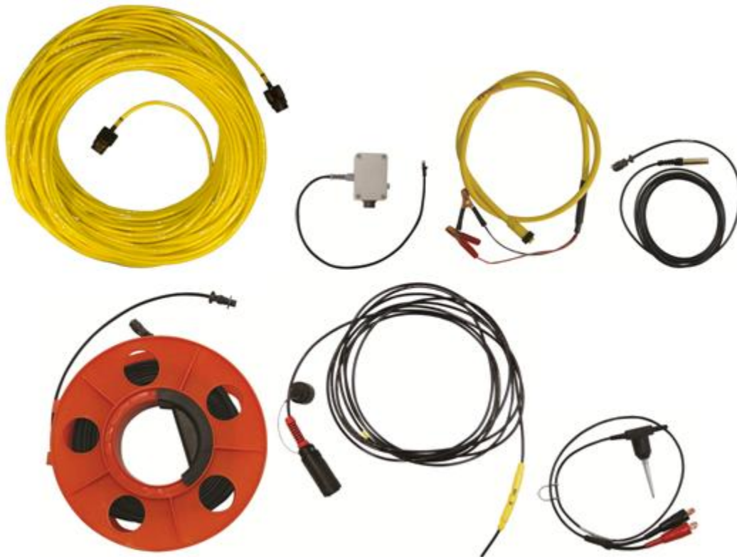
Figure B-3: Typical Geode accessories, clockwise from upper-left: digital interface cable, network interface box (NIB), power cable, hammer switch, trigger extension cable, geophone cable, geophone.
