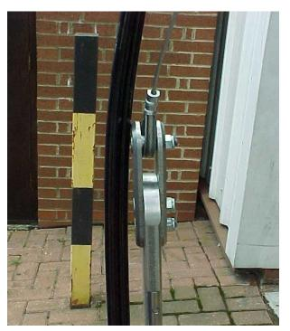
required to ensure no strands are broken as this could cause wear to the hose. It is also important to assemble in the correct way as indicated by the picture on the left. The nut on the cable bolt is shown to be on the opposite side to the hose, which is important as the striker assembly moves up and down in relation to the hoses during operation. This assembly configuration minimizes the potential for wear to the hose.
