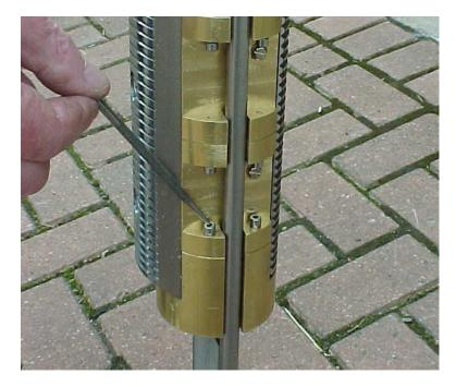
mechanical impacts may cause loosening of bolts employed in the hammer construction as illustrated. It is recommended that regular and routine inspection (before and after a survey) is carried out to the overall assembly. This will alert the operator to any issues which should be rectified before use or storage of the hammer. Failure to adhere to this may result in hydraulic leaks within the hammer body.
