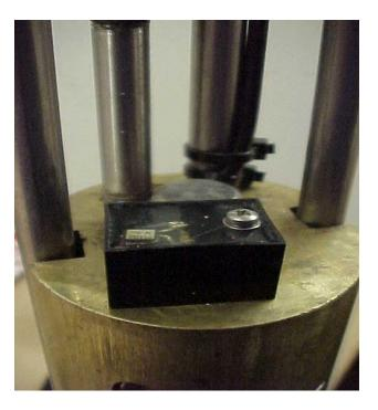
need to be attached to the hammer body with some care to ensure reliable operation and to protect the cable from damage by the operation of the sliding hammer. The switch has a short length of cable with a waterproof connector attached. Connection to the seismograph on the surface is by means of an extension lead, which has a waterproof connector that mates with the connector on the switch lead and a connector at the surface compatible with the seismograph.
