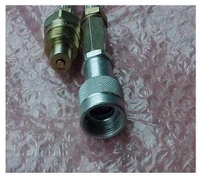
could prevent the ball valves closing when the couplings are separated resulting in leakage of hydraulic fluid. Allowing grit to enter the hydraulic fluid could result in expensive internal damage to the internal parts of the hammer.
