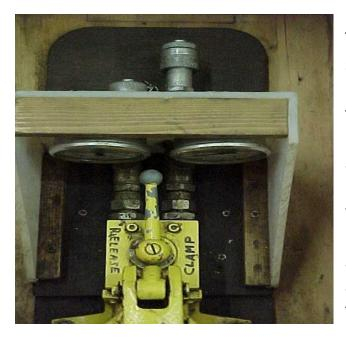
The shear wave hammer system employs a simple mechanical principle whereby the hammer is lowered into a borehole to the desired depth and is clamped in situ by means of a moveable plate which extends out from the hammer body. This plate is activated by a hydraulic pump at the surface, with fluid transferred by hose from the pump to hammer. The pump is
