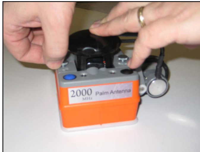
Figure 5: Re-secure the encoder assembly.
