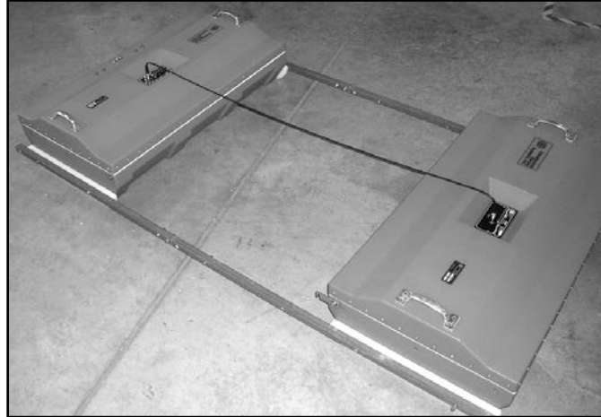
Figure 3: Hardware Setup for the 3207 Bi-Static using the co-axial transmit trigger cable.
