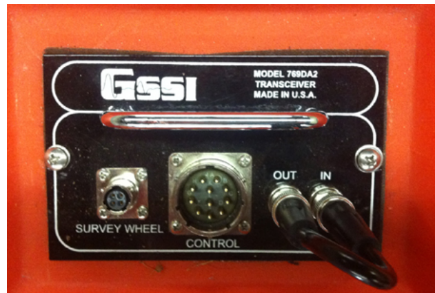
Figure 4: Model 769DA2 Setup for Mono-Static Mode.
