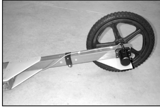
Figure 9: The Model 620 Survey Wheel.
