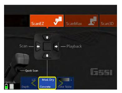
4 Once you have configured the XT, pull the trigger or select Scan from the handle keypad to begin collecting data.
