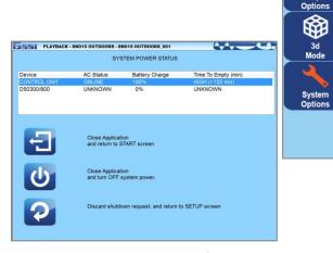
**Note**: If the system was not powered down properly and before the next time you power up, you must disconnect the battery on the antenna and then re-connect it. This will turn the antenna off, then back on. You can now power up normally.
