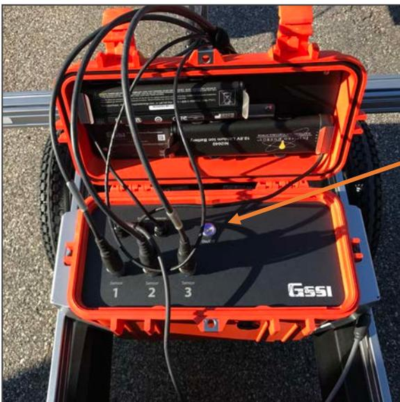
The final step is to press the power button on the orange concentrator box to power-down the sensors.
