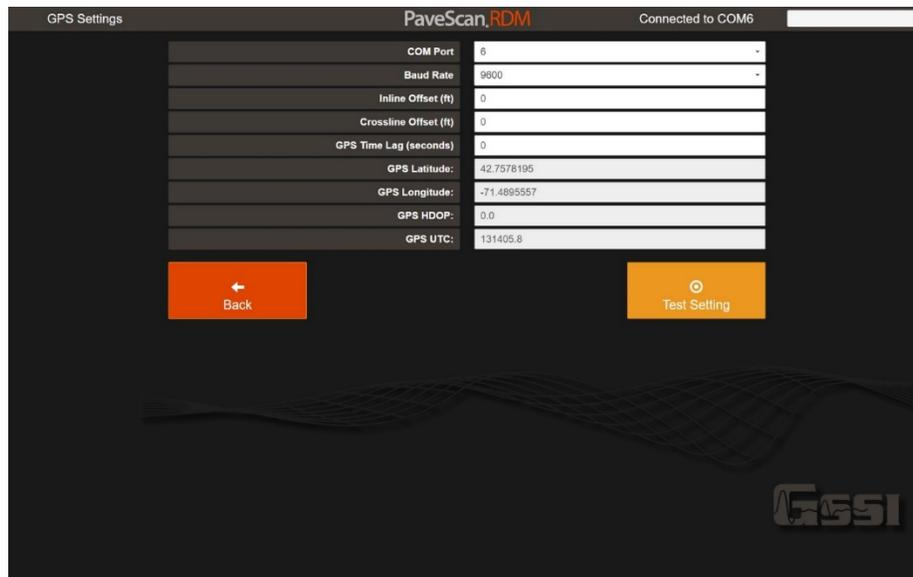
**COM Port:** The COM port the GPS is attached to. You may have to scroll through the different available COM ports to detect the COM port the GPS is attached to. Do this by selecting a COM Port, then pressing the **Test Setting** button and waiting 5 seconds.
