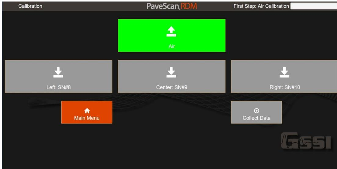
The image below indicates that the calibration procedure is ready to begin with the airwave measurement.
