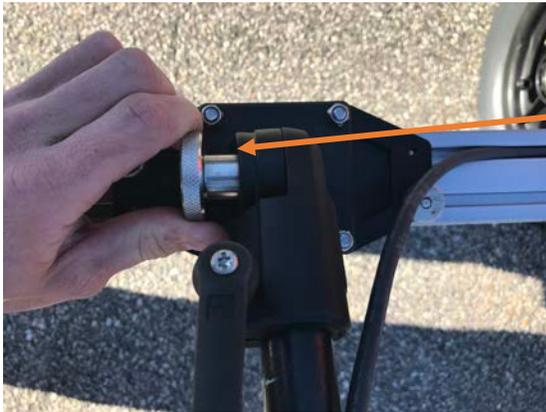
Loosen this thumbscrew, lift sensor arm, and then retighten prior to airwave measurement
