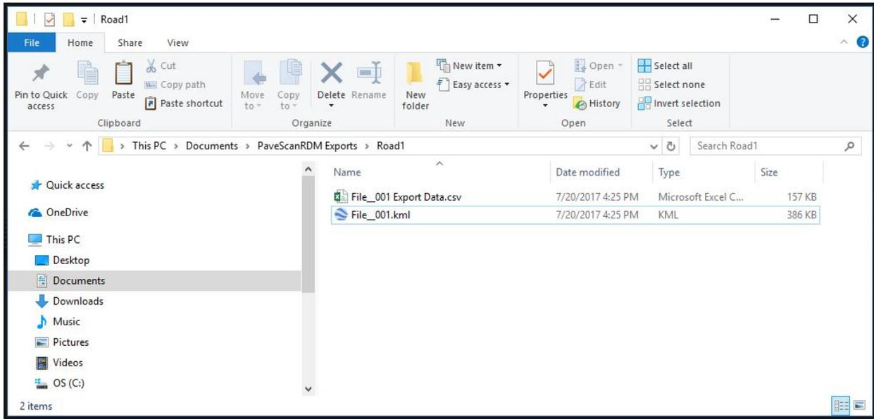
The exported file is an ASCII file containing a number of header lines containing project and file information followed by the exported data, which consists of comma separated values. You can choose to skip exporting the header lines by deselecting the Use Extended Header option in the Export Settings window (which is accessed from the Project Properties window). A portion of a typical exported file is shown below.
