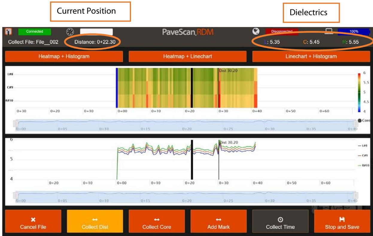
Clicking on the different buttons on the top of the window shows different combinations of windows.
