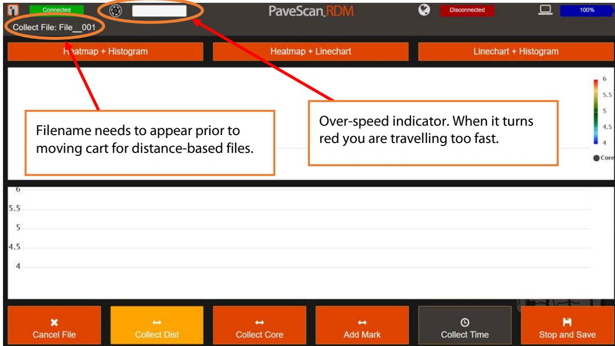
Filename needs to appear prior to moving cart for distance-based files.
