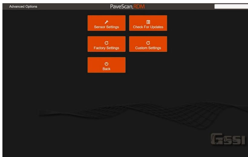
Select the Advanced button to check for updates or modify sensor settings. Sensor settings are not typically modified after they are entered the first time a sensor is attached to the PaveScan system.
