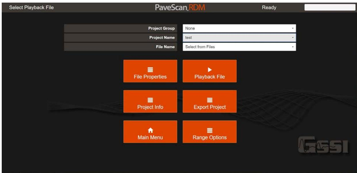
Select the desired Project and File from the dropdown lists, then press the Playback File button. Additional options in the Playback menu include:
