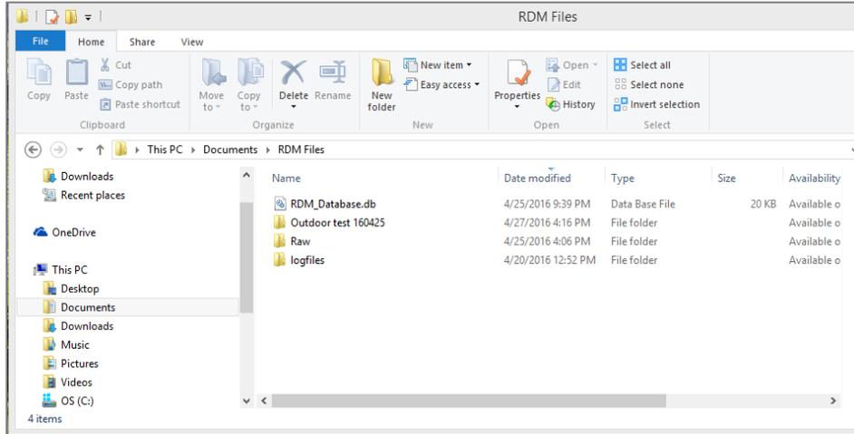
The software utilizes a SQLite database file to store the project and file information. The name of the file is “RDM\_Database.db.” The dielectric file data are stored in ASCII files in the “Raw” subfolder. The naming convention of the dielectric files is YYMMDDNN\_FN\_SN.txt
