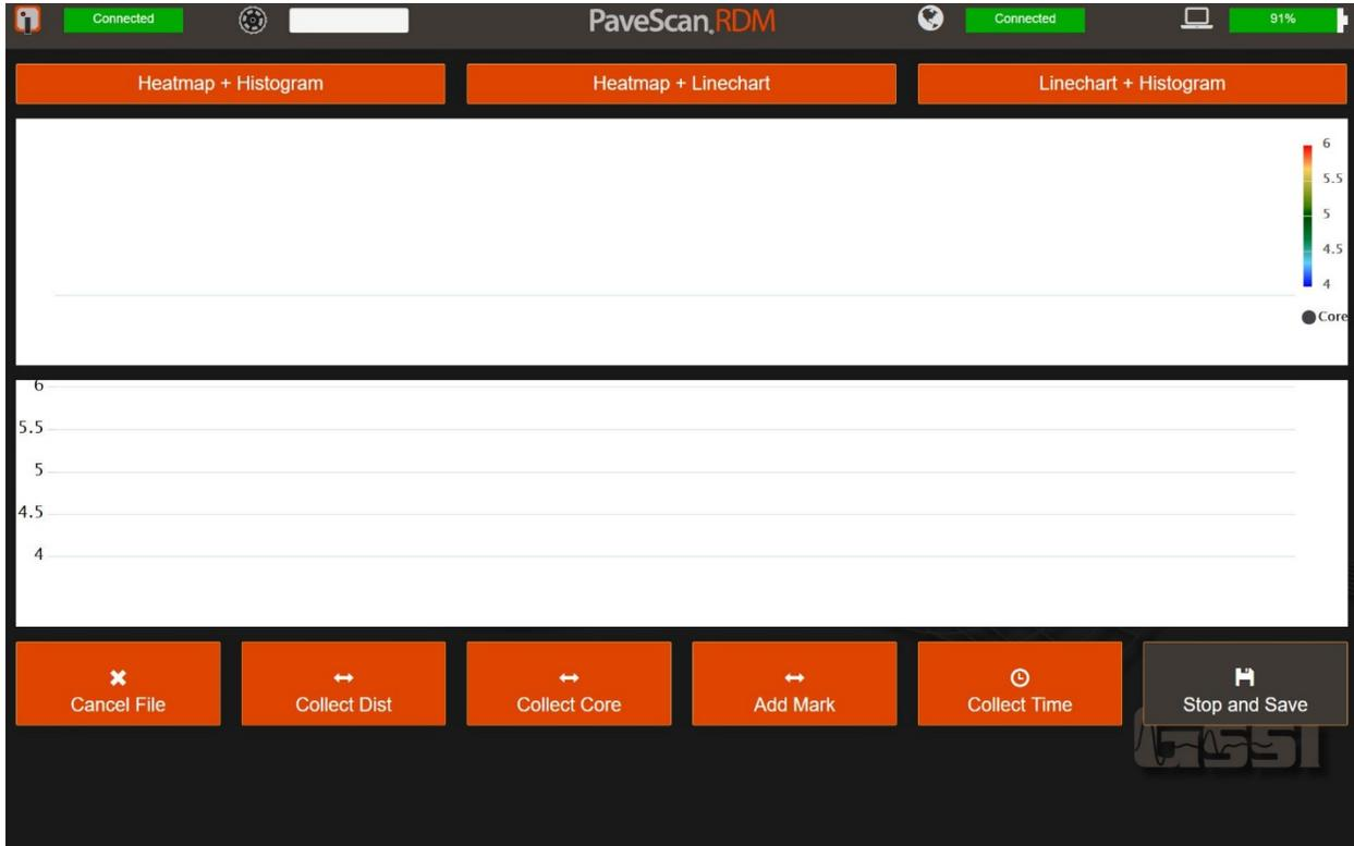
No data collection starts until either the Collect Dist, Collect Core or Collect Time buttons are pressed.
