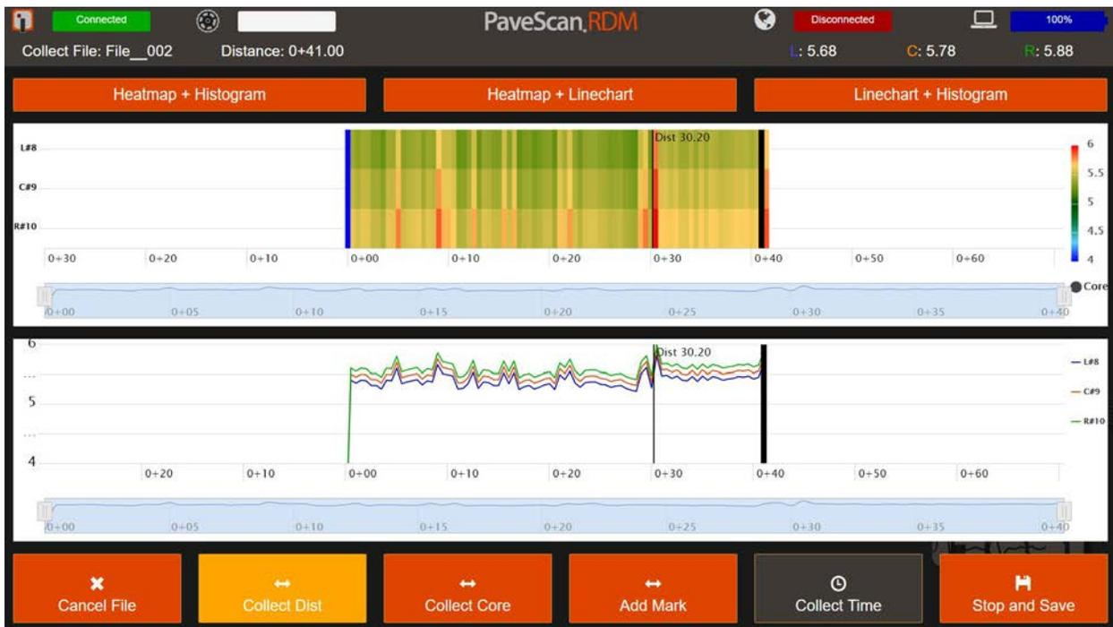
When backing up, the current distance and dielectrics associated with the sensor positions are indicated at the top of the window and the back-up location in the data is indicated by a large black bar.
