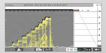
LifeLocator TRx screen example showing moving person (leg motion) at varying distances away from the sensor. Starting at 11m moving in 1m increments until 2m away from the sensor. The white line at the bottom of the data indicates presence of radio interference located at the site.
