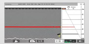
LifeLocator TRx screen example showing a breathing victim at 7m in depth, and breathing at a high rate. The red line on the left screen panel indicates position of victim, and the right screen panel shows breathing rate and depth of detection. The white line at the bottom of the data indicates presence of radio interference located at the site.
